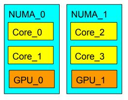
GPU\_0 can only be allocated with Core\_0 and/or Core\_1
