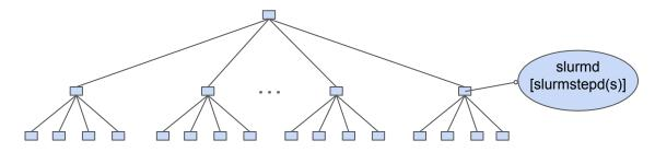
Configurable virtual network for communications (TreeWidth / TopologyParam)
