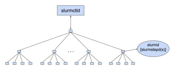
Configurable virtual network for communications (TreeWidth / TopologyParam)
